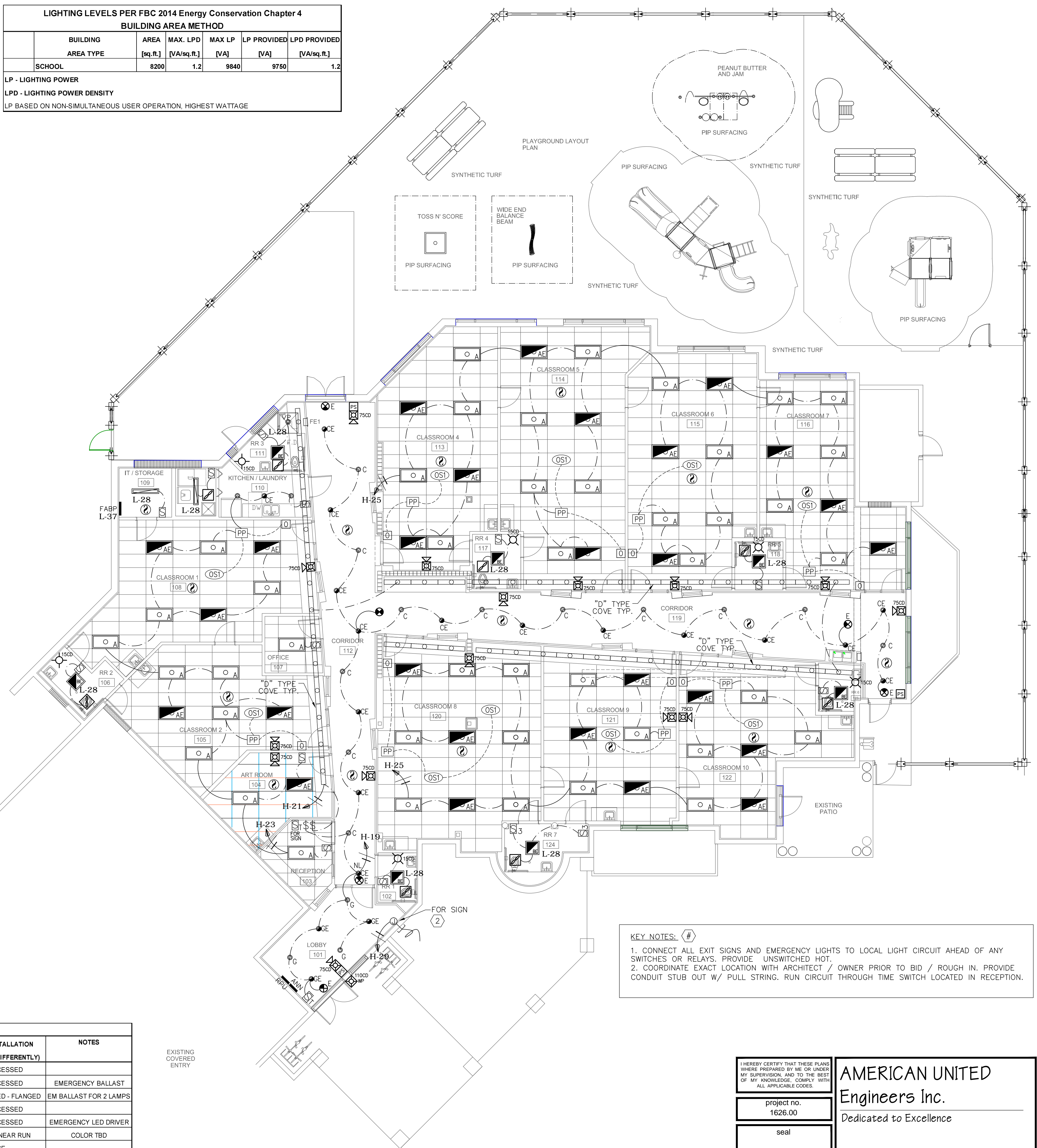
1ST FLOOR LIGHTING AND FA PLAN scale: 1/8" = 1'-0"
