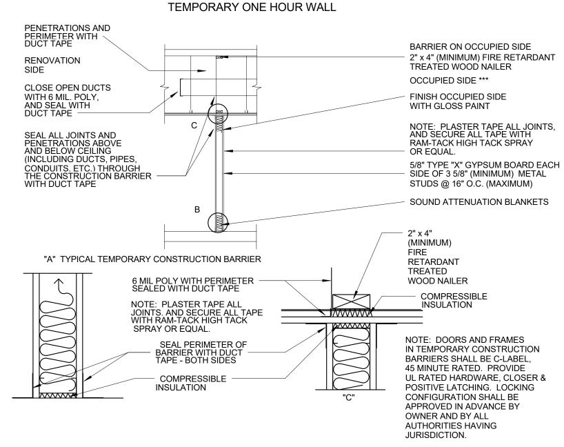
WALL TYPE- TEMPORARY ONE-HOUR FIRE BARRIER
