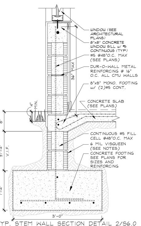
— DUR-O-WALL METAL REINF. @ 16" O.C. ALL CMU WALLS CMU BLOCK (SEE PLANS)  $_{-}$  8"x8" MONO. FOOTING  $\omega/$ (2)#5 CONT CONCRETE SLAB (SEE (PLANS) CONTINUOUS #5 FILL CELL @48"O.C. MAX - 6 MIL VISQUEEN (SEE NOTES) CONCRETE FOOTING SEE PLANS FOR SIZES AND REINFORCING 21-01 TYP. STEM WALL SECTION DETAIL 3/56.0
