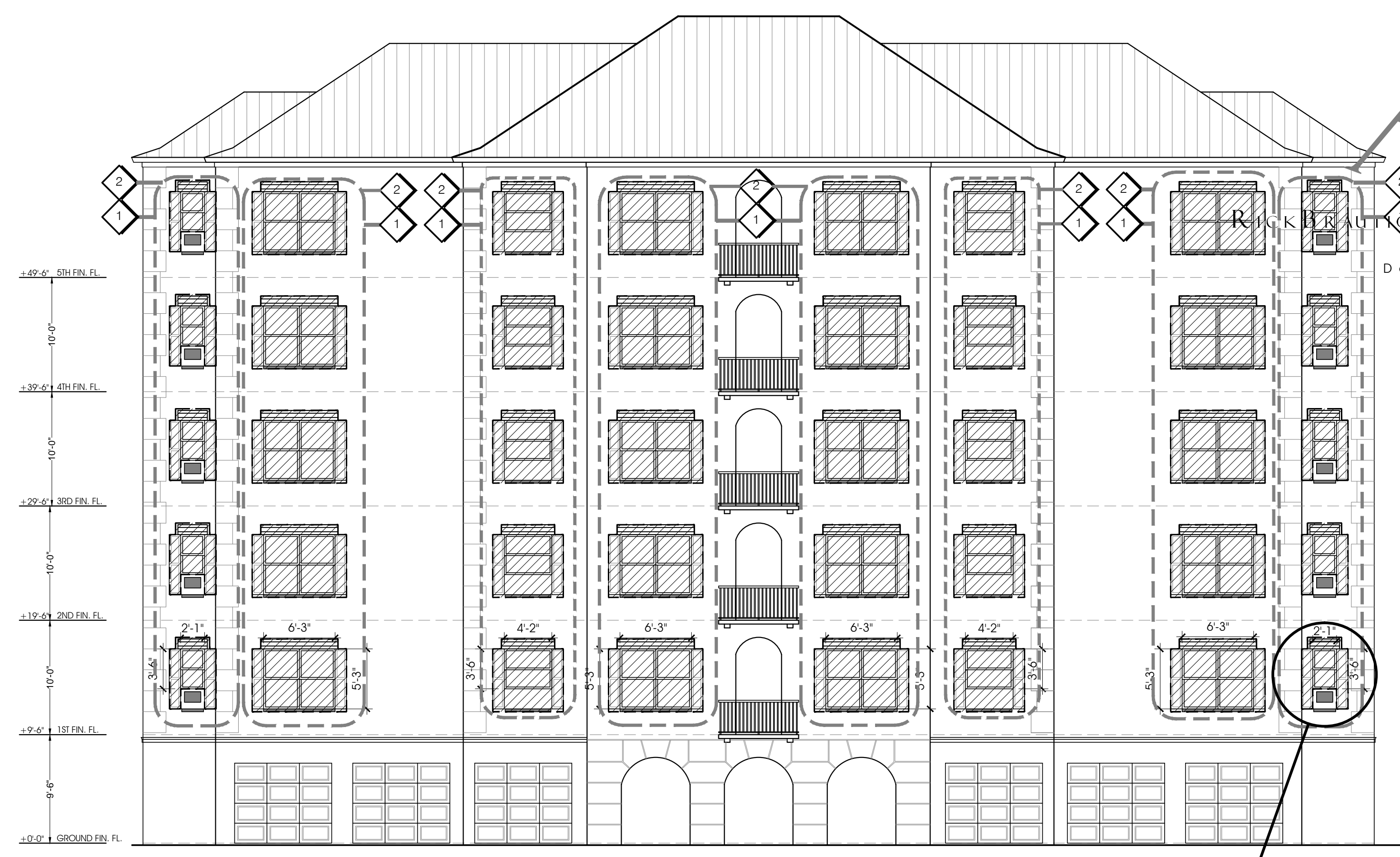
Front Elevation 1/8" SC NOTE: EXISTING BALCONIES/ RAILINGS / SGD ETC. TO REMAIN UNALTERED (TYP.)
