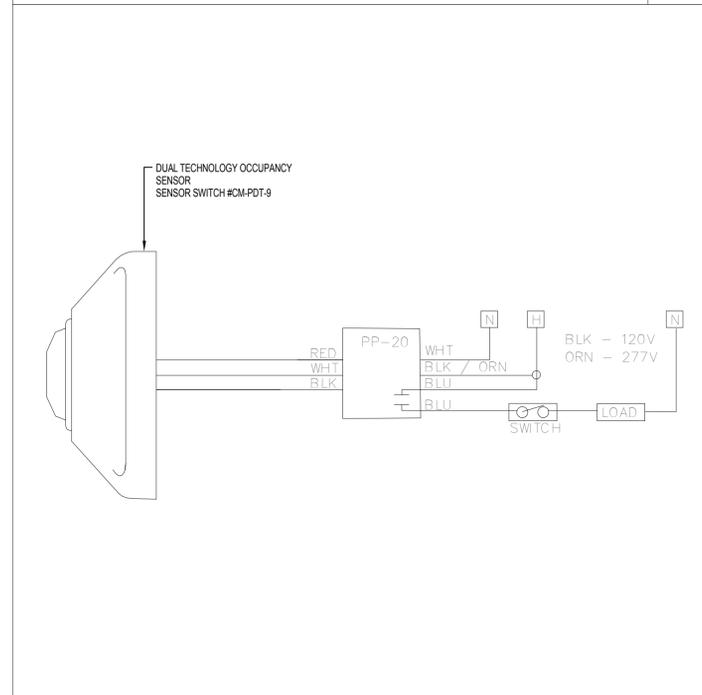
**TYPICAL OCCUPANCY SENSOR WIRING**
