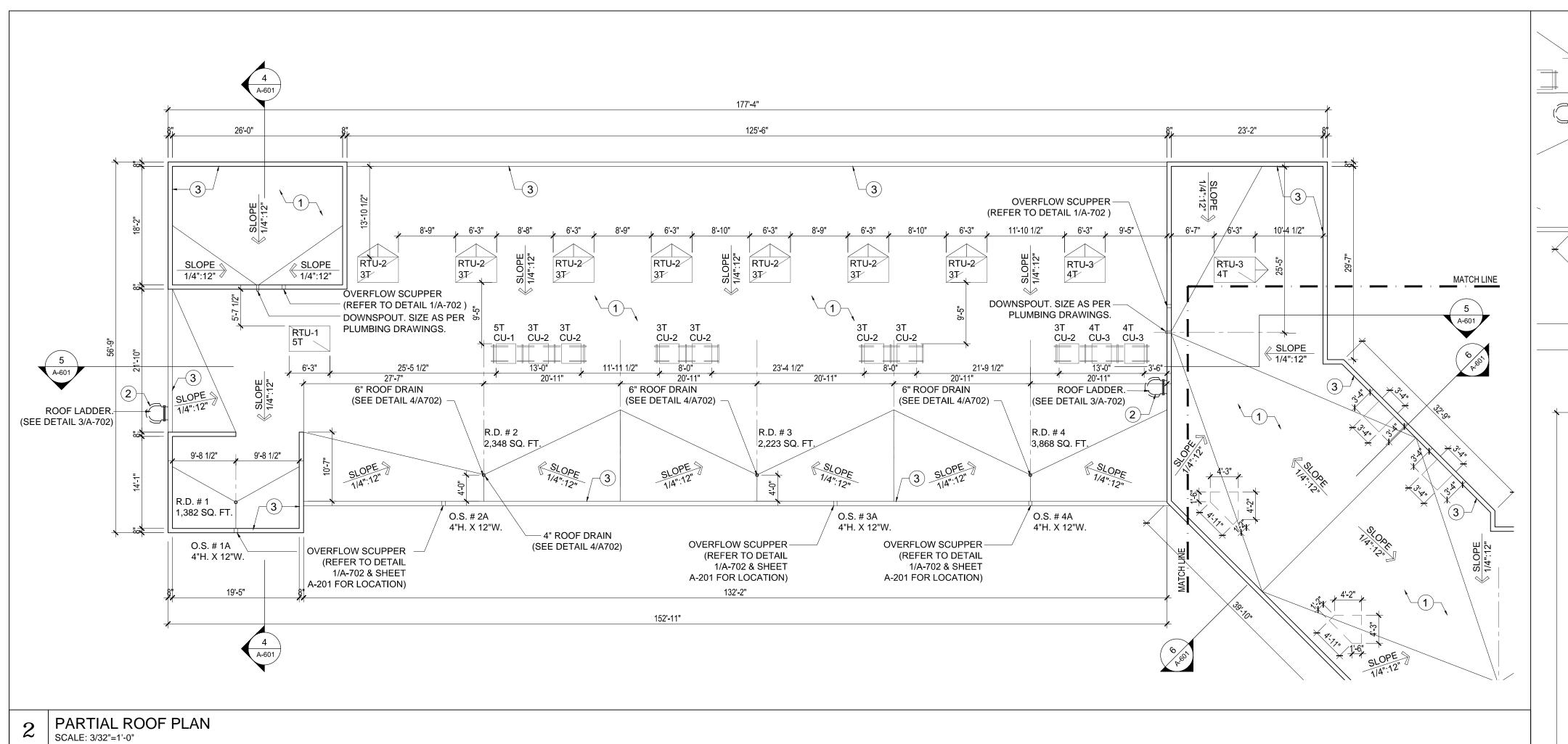
**GENERAL ROOF NOTES:** 1. SUBMIT ROOFING SHOP DRAWINGS FOR REVIEW AND APPROVAL BY ARCHITECT PRIOR TO SUBMITTAL TO BUILDING DEPARTMENT. SYSTEM SHOP DRAWINGS SHALL INCLUDE FLASHING DETAILS FOR ALL CONDITIONS.
