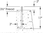
(4) 3/4"-10NC Galv. Stl. Anchor Bolts, AASHTO M314-90 Grade 55, 10" Of Threaded End Galv. Per ASTM A153. (4) 3/4"-10NC Galv. Stl. Hex. Nuts (4) 3/4" Galv. Stl. Lockwashers
