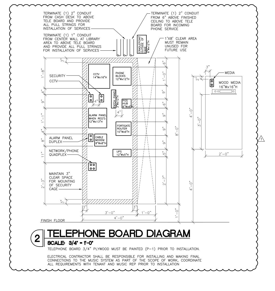
TENANT TELCO VENDOR TO DO ALL CONNECTION / TERMINATION FOR ALL TELEPHONE JACKS. TELEPHONE COMPANY BRINGS LINE TO TELEPHONE BOARD IN TENANT SPACE. IT IS THE RESPONSIBILITY OF TELCO VENDOR TO COMPLETE INSTALLATION OF TELEPHONE LINES, JACKS, AND PHONES FROM TEL. BOARD IN TENANT SPACE TO POINT OF TERMINATION.
