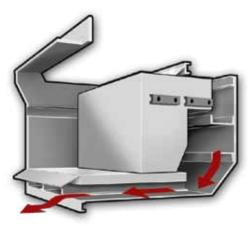
The Qwik Clean<sup>®</sup> Tank feature, standard on all RJ-250SC compactors, funnels any liquid seepage which can occur during compaction into an enclosed area underneath the charge box floor. The liquid is automatically discharged at the disposal site, in effect flushing the container and the area behind the ram. The 12-inches (305mm) high, 750-gallon (2839 liters) capacity sump area is designed to provide easier hook access for roll-off drivers.
