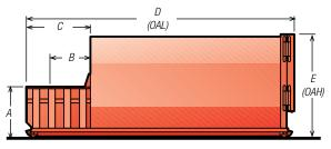
Dimensions not shown: 8' 4¼" (2543mm) Overall Width Ground Roller Widths: 61¼" (1569mm) Inside Rollers 67½" (1712mm) Roller Centers 72½" (1851mm) Outside Rollers
