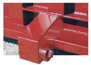
The **StreamLine** option enables excess liquid to be drained from the container, reducing net payload weight and significantly reducing hauling costs. Liquid is routed to four interconnected 4" (101.6mm) drain outlets located at each corner of the StreamLine unit. Connection can be made to a hose, piping, or a pump.
