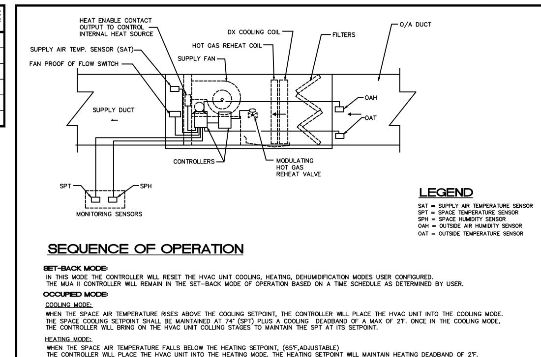
ONCE IN THE HEATING MODE, THE CONTROLLER WILL CLOSE A CONTACT TO ENABLE THE HEATER TO MAINTAIN THE SPT AT ITS SETPOINT.
