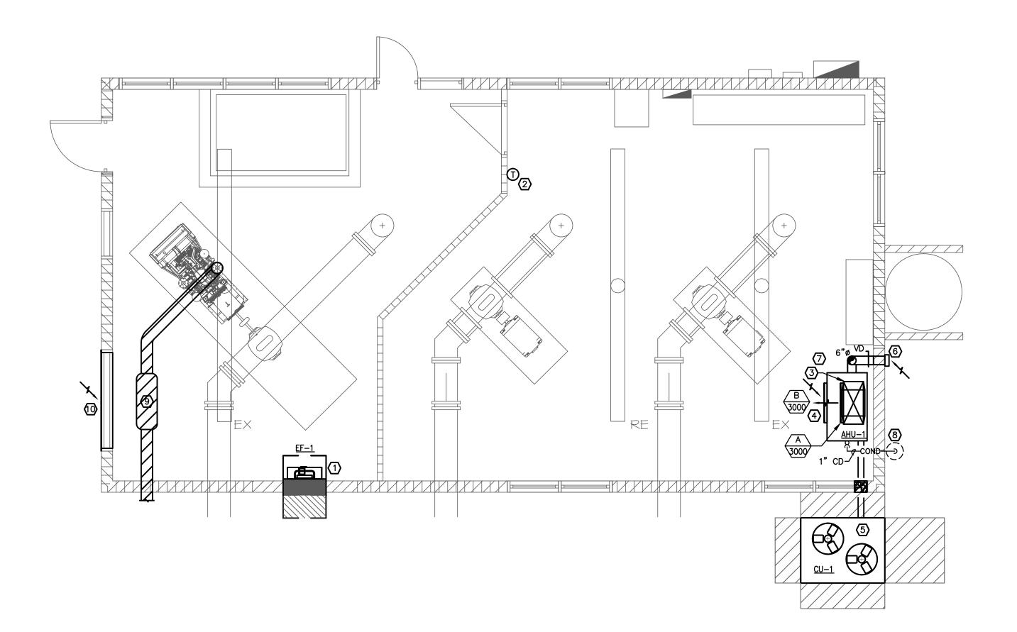
PLAN KEY NOTES INFORMATION. 30"x14" DISCHARGE PLENUM. 6"ø OUTSIDE AIR INTAKE WALL-CAP (GREENHECK WC-8 OR APPROVED EQUAL). PROVIDE PLENUM. PROVIDE CONDENSATE DRYWELL. FIELD COORDINATE EXACT LOCATION WITH OWNER/ARCHITECT. EXISTING DIESEL EXHAUST PIPE TO REMAIN. EXISTING INTAKE LOUVER TO REMAIN.
