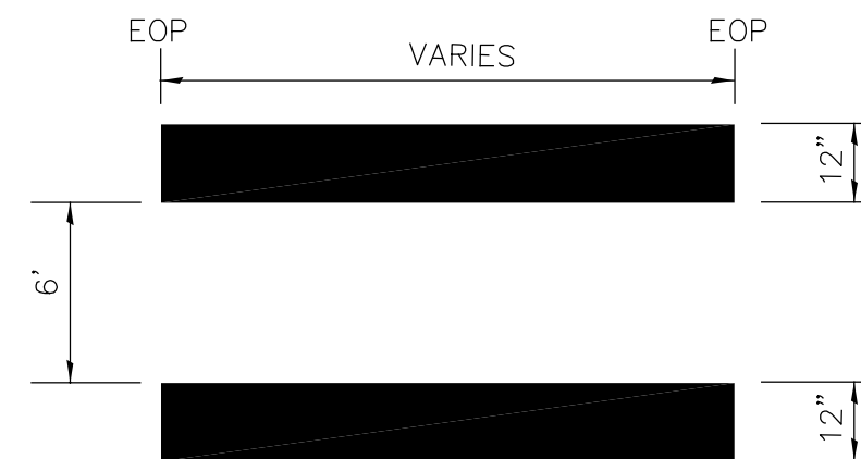
5 SOLID WHITE CROSSWALK / TRAFFIC CALMING DETAIL NTS
