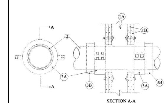
. Wall Assembly — The 1 or 2 hr fire—rated gypsum wallboard/stud wall assembly shall be constructed of the materials and in the manner described in the individual U300 or U400 Series Wall or Partition Design in the UL Fire Resistance Directory and shall include the following construction features:
